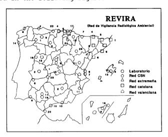
These stations are located in the same places that some National Weather Institute automatic stations. So, the meteorological parameters (air temperature, relative humidity, wind direction and speed, rain intensity and air pressure) are also received.
