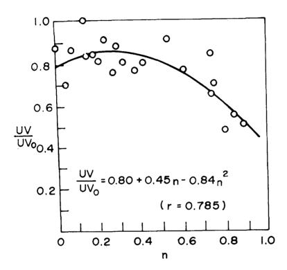
FIG. I. RELATIONSHIP BETWEEN RATIO OF ACTUAL TO CLEAR SKY SOLAR UV RADIATION (UV/UVO) AND CLOUD COVER IN FRACTION (n) (BOMBAY 1986-87)
