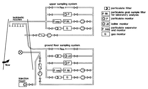
Fig. 2 NPP-Muehleberg backfited redundant stack effluent sampling and measurement system
