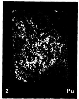
Sea Spider Maia squinado (Channel), Digestive gland. (200  $\mu$ m full horizontal scale) Ion probe images obtained from the same area (RIBER MIQ 156), 1:  $^{40}$ Ca $^+$ ,2: $^{239}$ Pu $^+$ Elements appear as bright points in the biological section.
