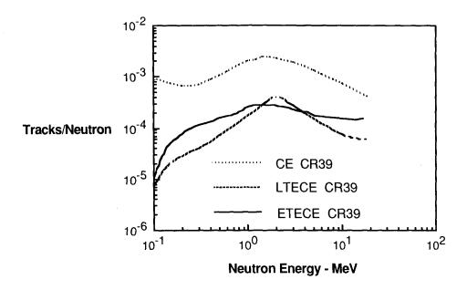
1. Comparison of typical CR39 neutron energy responses using chemical etching (CE), room temperature electrochemical etching (LTECE), and elevated temperature  $(60^{\circ}\text{C})$  electrochemical etching (ETECE).
