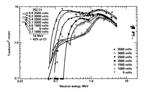
2. Illustration of the voltage dependent ETECE CR39 neutron energy response for a 5 hour, 60 Hz etch, using a fixed 3000 volt, 2 kHz ECE post etch (approximately 30 minutes).
