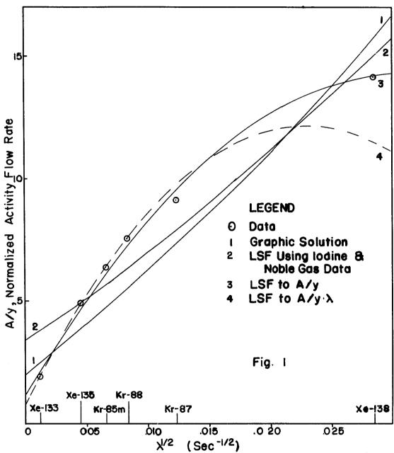
Noble Gas Activity Flow Rates at the Steam Jet Air Ejector of an Operating BWR
