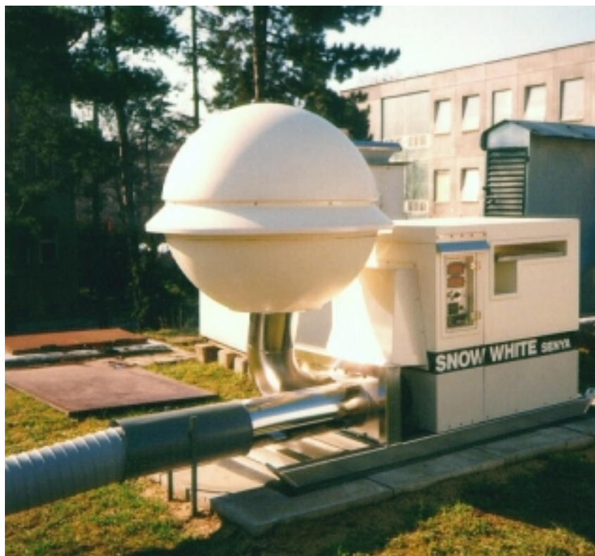
Fig.2: Aerosol sampler “Snow White” with the flow rate of 900 m 3 /h.
