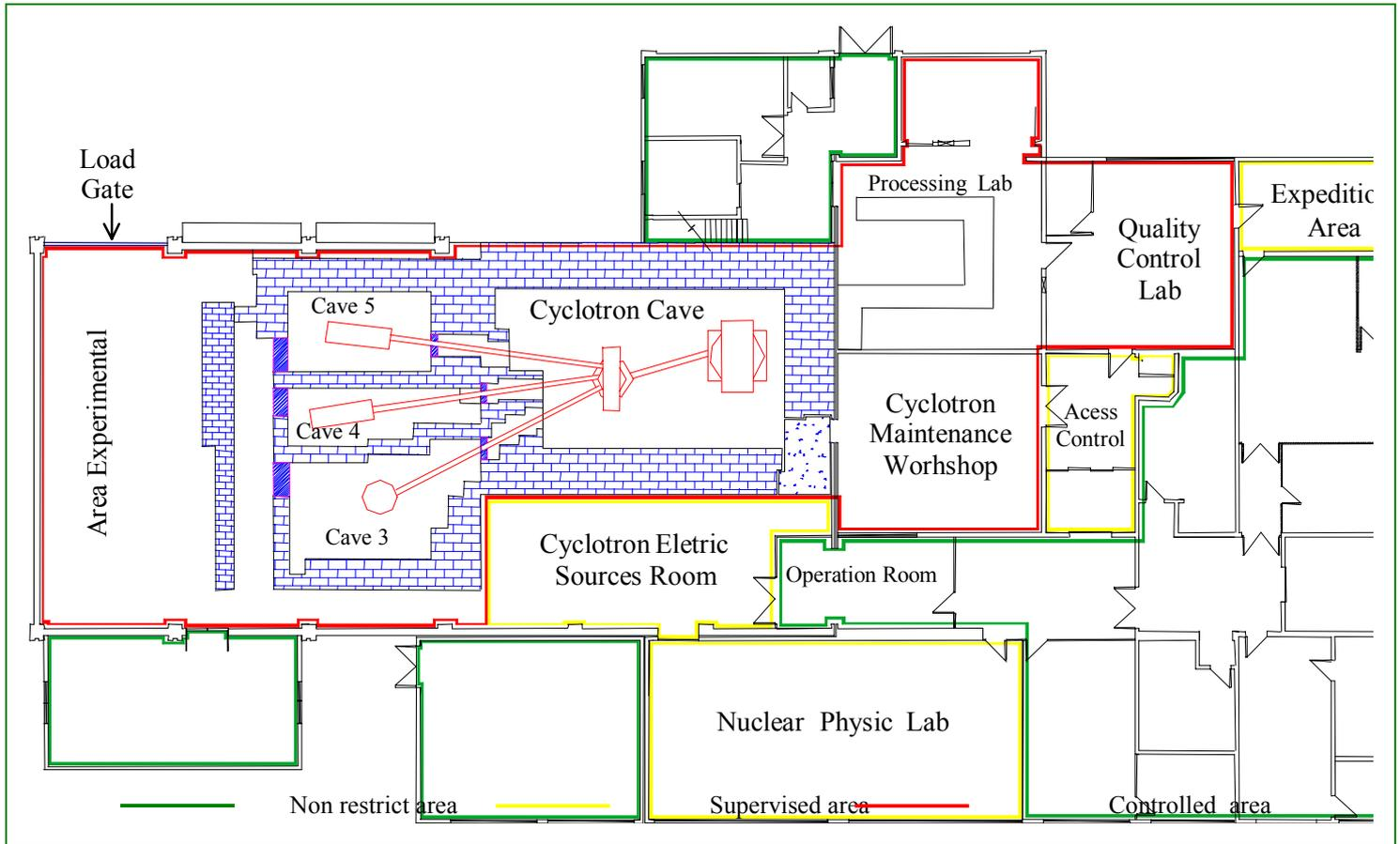
Figure 1: Layout of the main existent facilities in the 1<sup>st</sup> floor of the IEN Cyclotron installations building
