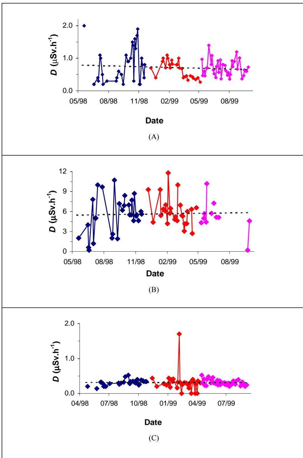
Figure 3: Gamma dose rates ( $D$ ) measured in the Cyclotron and Kipros system operator position (A); external area close to the load gate of the Cyclotron experimental area (B); and in the internal non restrict areas of the 1<sup>st</sup> floor of Cyclotron installations (C). Operation to 10  $\mu$ A (blue line), 15  $\mu$ A (red line) and 20  $\mu$ A (purple line). Black stippled line: tendency line
