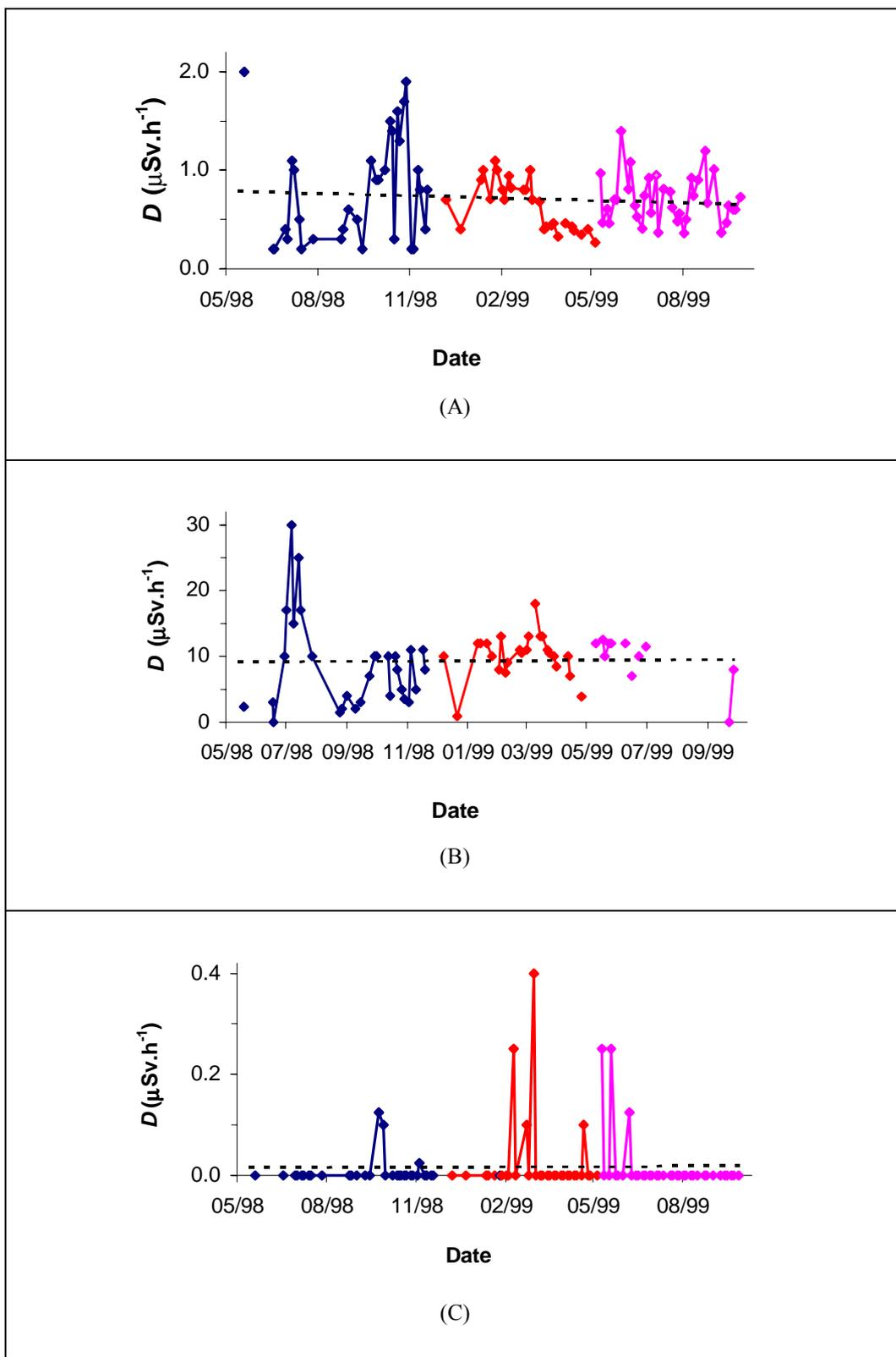
Figure 2: Neutrons dose rates ( $D$ ) measured in the Cyclotron operator position (A); external area close to the load gate of the Cyclotron experimental area (B); and in the internal non restrict areas of the 1<sup>st</sup> floor of Cyclotron installations (C). Operation to 10  $\mu$ A (blue line), 15  $\mu$ A (red line) and 20  $\mu$ A (purple line). Black stippled line: tendency line
