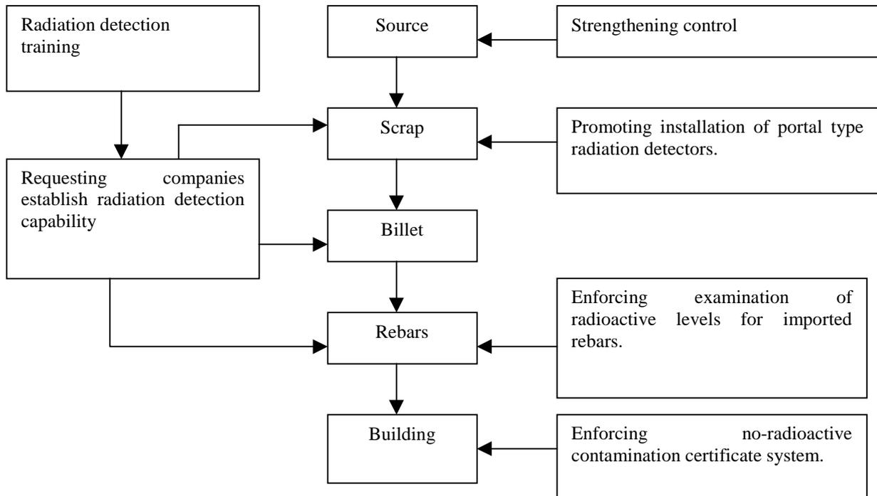
Figure 2. Measures to prevent rebars from being radioactively contaminated.
