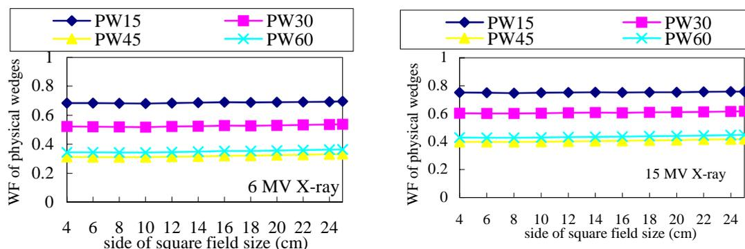
**Fig 1. The wedge factors versus the sides of square field sizes for physical wedge for 6- and 15-MV beam.**
