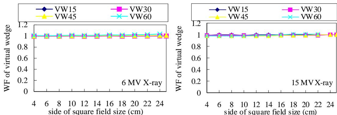
**Fig 2. The wedge factors versus the sides of square field sizes for virtual wedge for 6- and 15-MV beam.**
