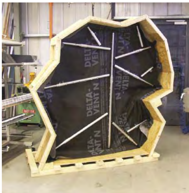
Figure 4: First idea (left) and prototype installed in a wooden model of an underground gallery (right) of the Express - Air Screen - System (EAS) for miners
