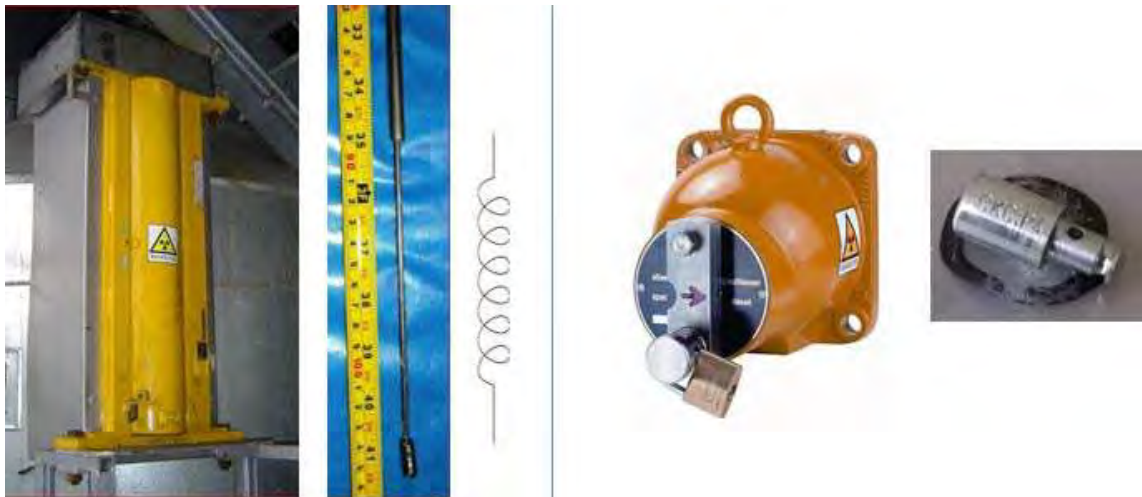
Figure 5: Line (left) and point (right) source gauges for industrial measurement (photos courtesy J.A. Tompkins, IAEA)
