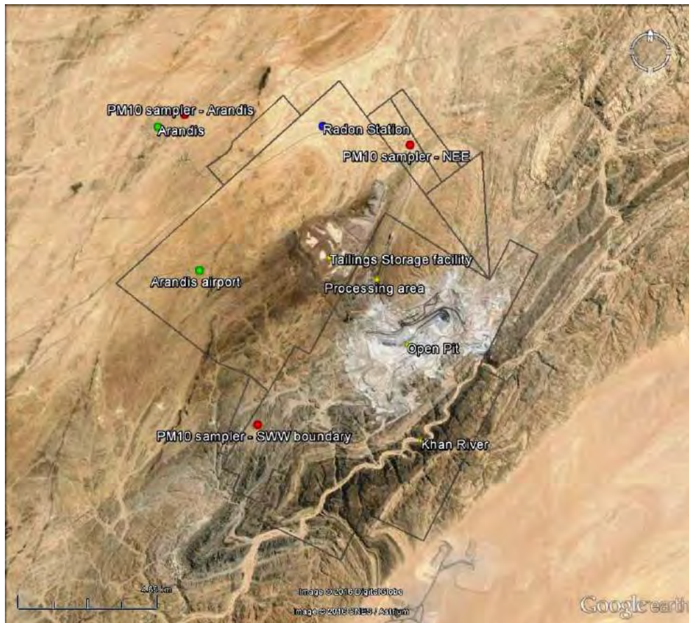
Figure 3: Rössing mine in relation to the locations of PM10 samplers (red) and radon monitoring station (blue)
